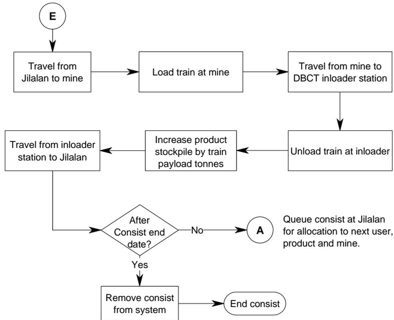
Figure A2. Flowchart for sending a train to a mine
