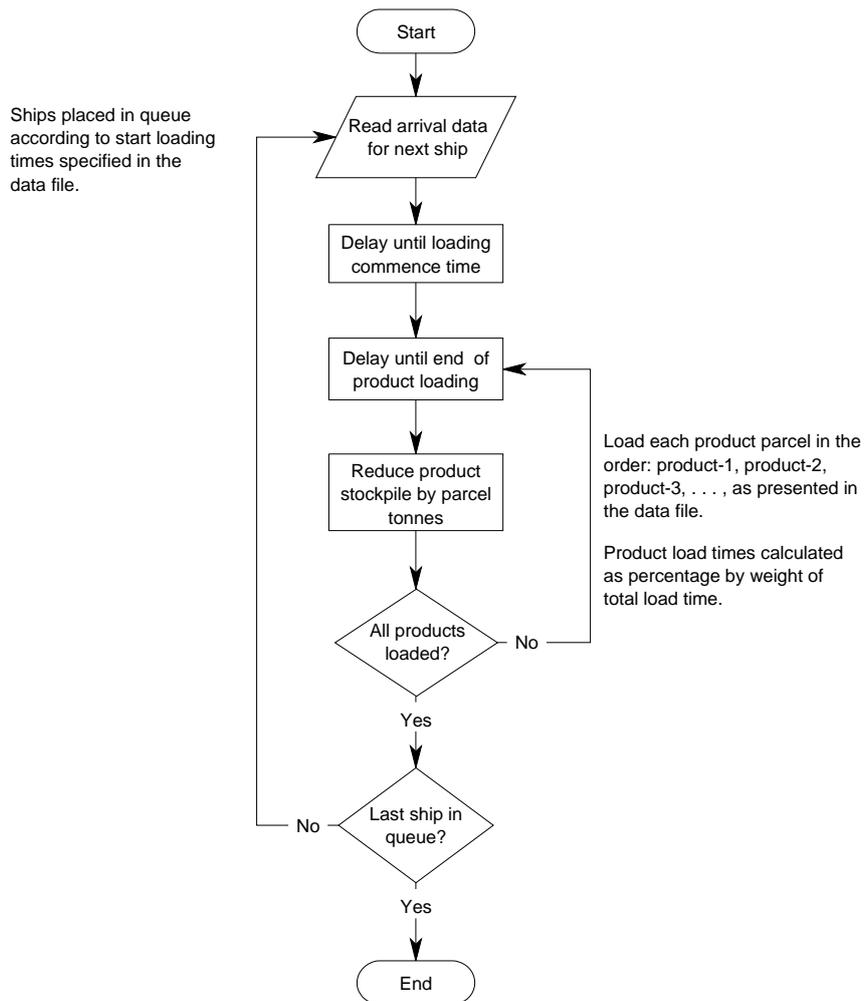
**Figure A1.** Flowchart for loading ships
