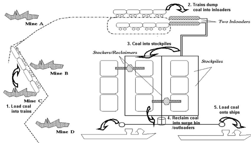
**Figure 2.** Transporting Coal from Mine to Ships
