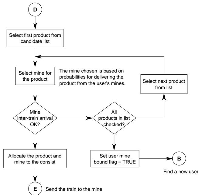
Figure A3. Flowchart for allocating a mine to a consist
